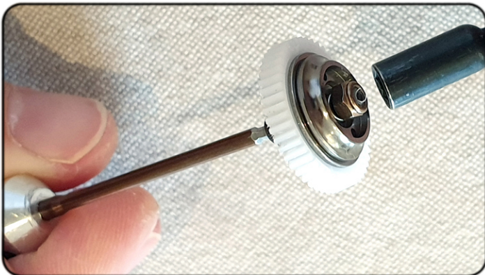
ADD LOCKNUT TO DIFF ASSEMBLY WITH SPRING WASHER BEHIND IT
