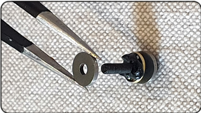
ADD WASHER TO COMPLETE THRUST RACE ASSEMBLY
