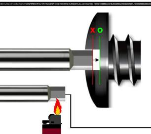
TENCACE DRIVER FULLY INTO SCREW SOCKET
